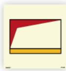
High expansion foam supply trunk (outlet) [SIS039]
