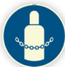
Secure gas cylinders
