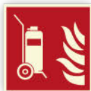
Wheeled fire extinguisher [FES006]
