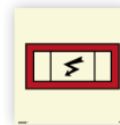
Emergency switchboard [SIS050]
