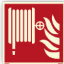
Fire hose reel [FES002]
