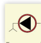
Emergency bilge pump
