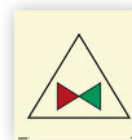
Remote control for fire pump valves [SIS032]
