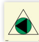
Remote control for bilge pump(s) [SIS028]
