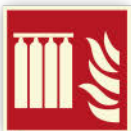
Fixed fire extinguishing battery [FES005]
