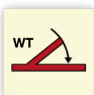
A class self-closing watertight fire door
