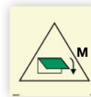
Remote control closing device(s) for ventilation inlet and outlet (Machinery) [SIS020]
