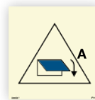
Remote control closing device(s) for ventilation inlet and outlet (Accommodation) [SIS019]
