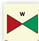
Fire main section valves [SIS035]
