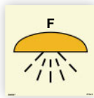
Space or group of spaces protected by a foam fire-extinguishing system [SIS043]
