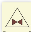
Remote control for fuel oil valves [SIS030]
