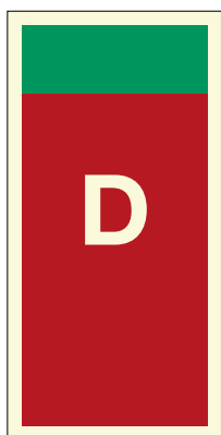
Supplementary sign for extinguishing media: Drencher
