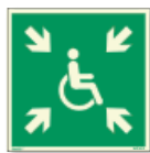
Evacuation temporary refuge [E024]
