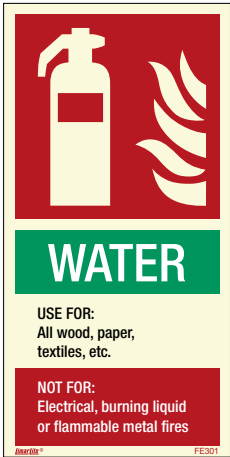
Water fire extinguisher instructions
