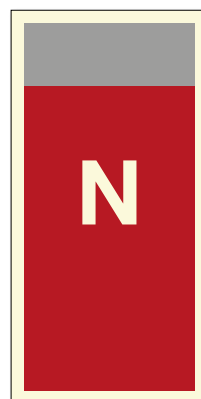
Supplementary sign for extinguishing media: Nitrogen
